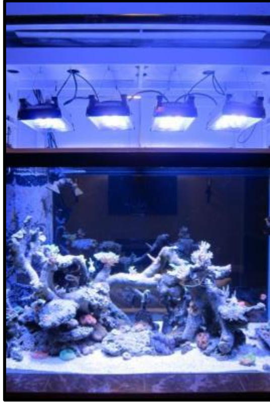
Figure 34: LED Fixture over 150-gallon Aquarium
