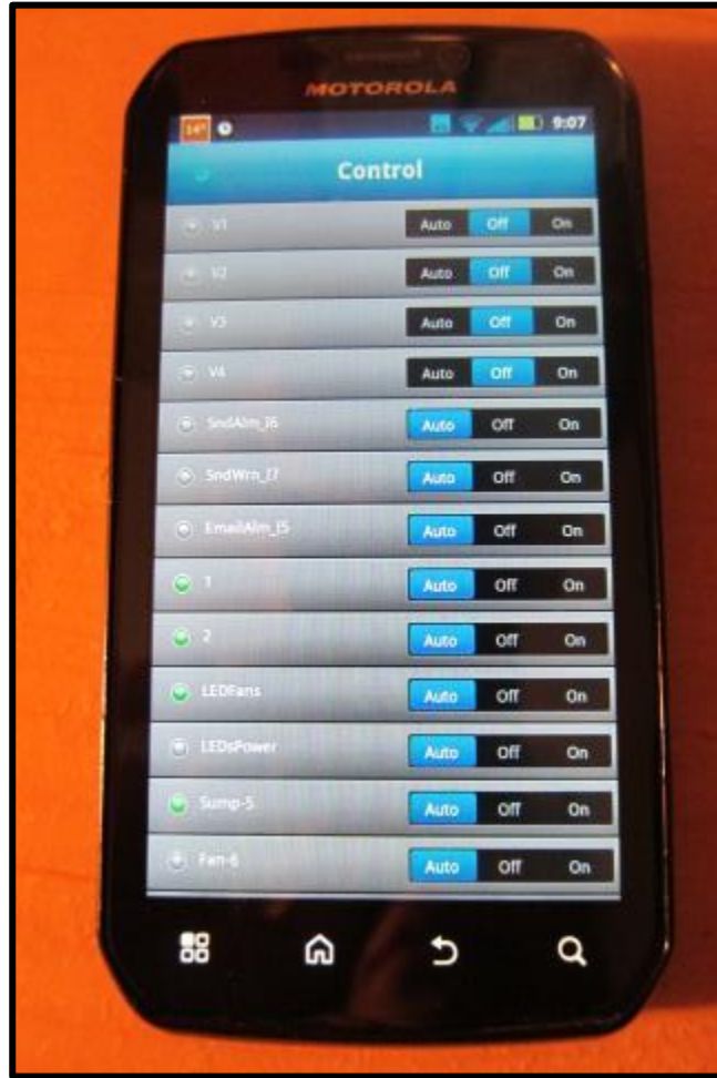
Figure 37: Cell Phone Control Panel
