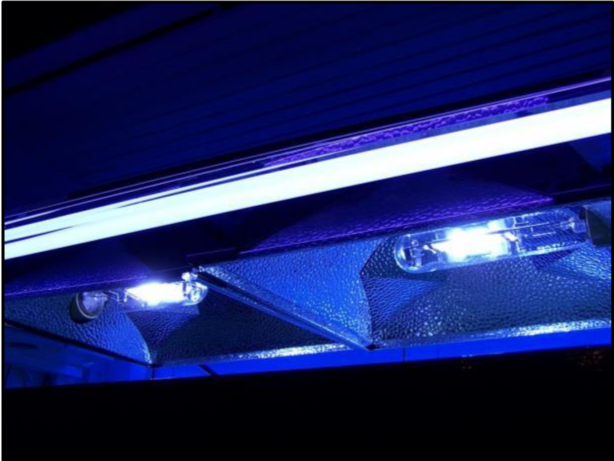
Figure 1: Author's Lighting System; Two x 400W MH and Two x 54W T-5
