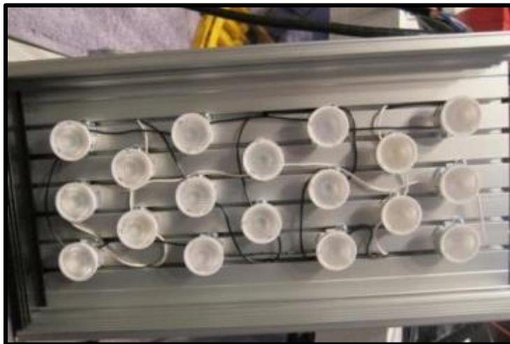
Figure 103: LEDs Covered in Optics
