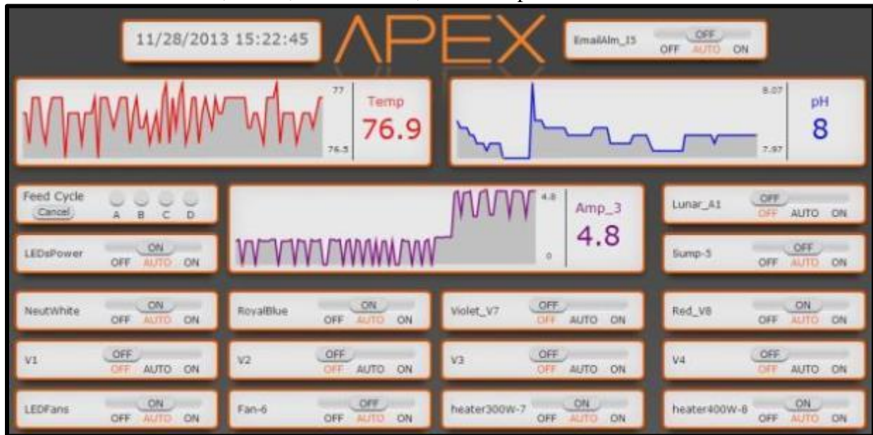
Figure 35: Remote Neptune Apex Control Panel
