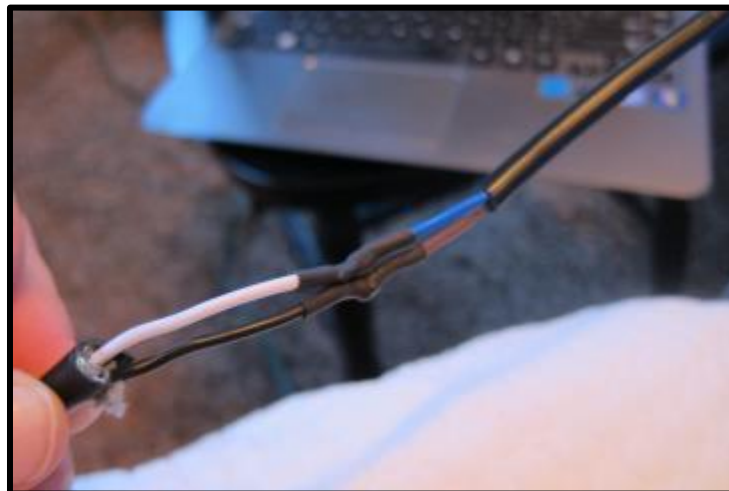
Figure 79: Adding the AC Power Cord to the Meanwell Drivers
